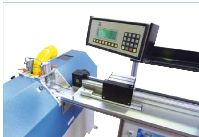
Exenso Basic with deposit tray for GMF measuring calipers, set up with a glazing bead saw.
